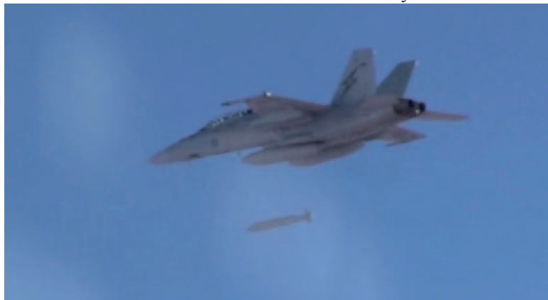
Release of AGM-154C Joint Standoff Weapon from a Super Hornet
